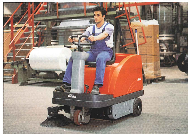
Hako-Jonas 900 E: For exhaust-free indoor applications with electric drive and various types of battery systems.
